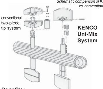
Schematic comparison of KENCO Uni-Mix System vs. conventional two-piece tip system
